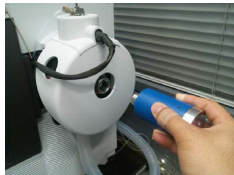
Step 2: Insert the capillary into the probe, and insert the probe into the ionization source.
