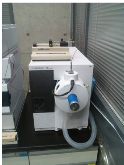
Figure 3. Overview of the ASAP/MS system with an infusion pump installed to introduce the calibrant used for accurate mass calibration by MassWorks.
