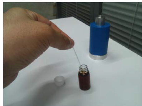
Step 1: Apply a sample to the capillary.
